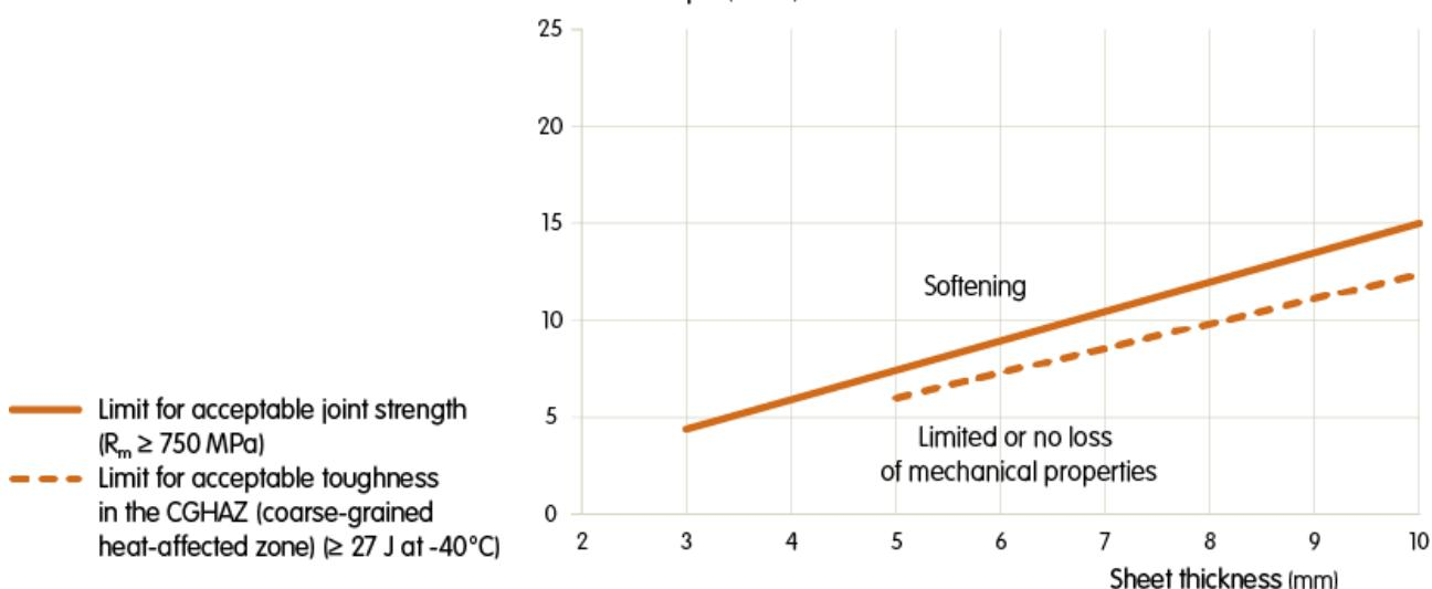
Recommendations for selecting the suitable heat input for MAG welding of Armstrong™ 700MC grade.
