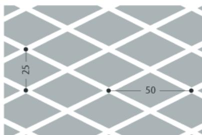
The height of the checkerboard/diamond pattern is between 1 and 2 mm.
